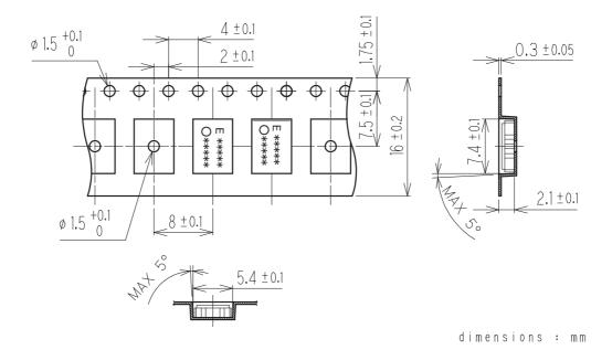
Carrier tape Top tape Carrier tape Components **MIN 100** MIN 160 Tape trailer MIN 400 Tape leader 10.5±0.4 2±0.5 ø 180 <sup>+0</sup> -3 \$ 60 +1 13 ± 0.2 ₩ Quantity 1000pcs/Reel 17 ±0.3 19.4 ±1 dimensions : mm
