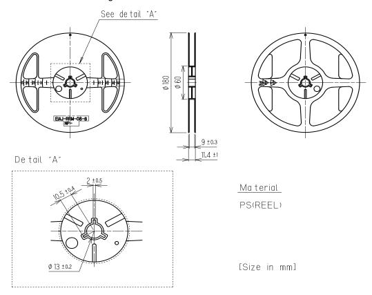
Tolerance for all measurements are +/-0.1mm unless otherwise stated.
