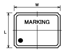
Marking TBD Material Ceramics(base) Au coated nickel(terminal) Fe-Ni-Co(lid)
