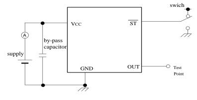
\*Current consumption under the disable function should be = GND.
