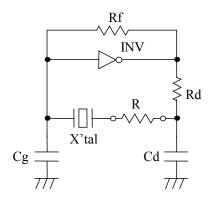
1) Connect the resister(R) to the circuit in series with the crystal unit.
