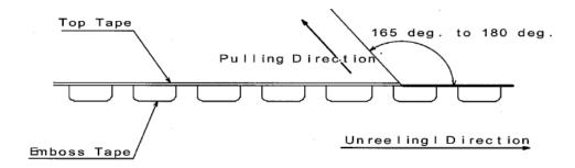
(a) angle : cover tape during peel off and the direction of unreeling shall be  $165^{\circ}$  to  $180^{\circ}$ .
