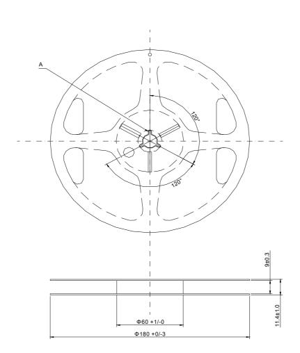
Material:Polystyrene (Conductivity) unit:mm
