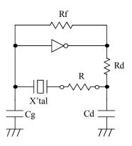
(1) Connect the resister (R) to the circuit in series with the crystal unit.
