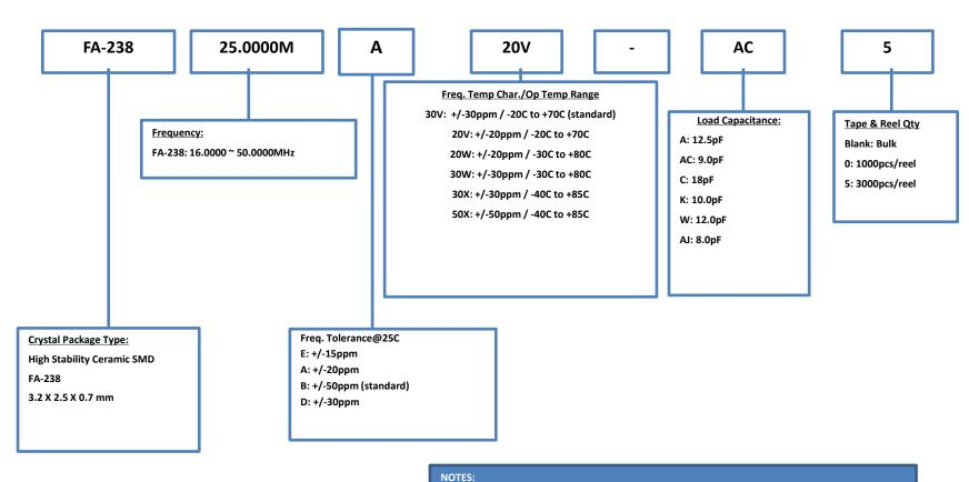
If you require frequency, tolerance, frequency temperature characteristics over temperature and load capacitance values other than the above listed, please contact your Epson representative for assistance.
